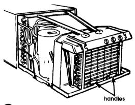
**6** Pull on handles; slide air conditioner out of cabinet and place on cardboard.
